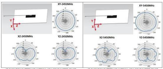
2D RADIATION PATTERN OF ANTENNA AT 2.45GHZ IN FREE SPACE
