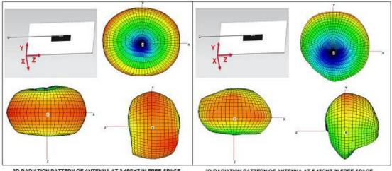
3D RADIATION PATTERN OF ANTENNA AT 2.45GHZ IN FREE SPACE
