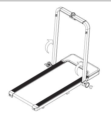
Snap the Armrest Group (3) into the Column (2). Note: Please patiently insert the armrest horizontally into the column to the end, and press down to lock A and B.
