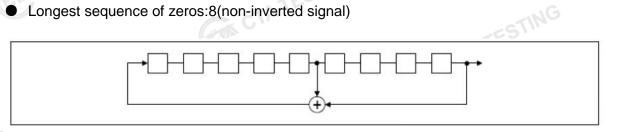
Linear Feedback Shift Register for Generation of the PRBS sequence
