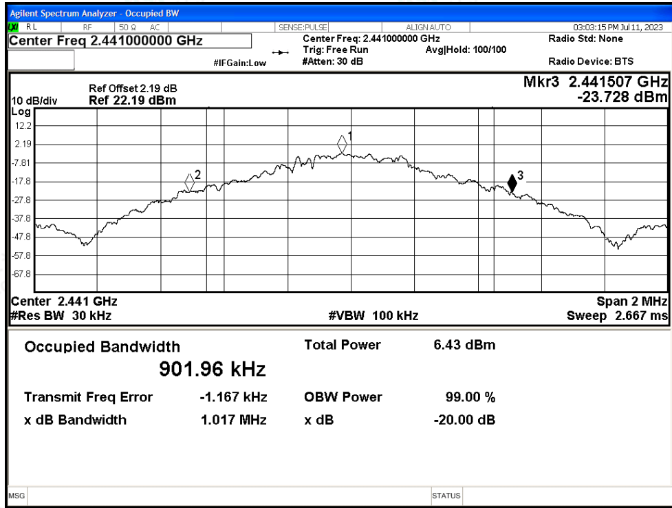
-20dB Bandwidth NVNT 1-DH5 2441MHz Ant
