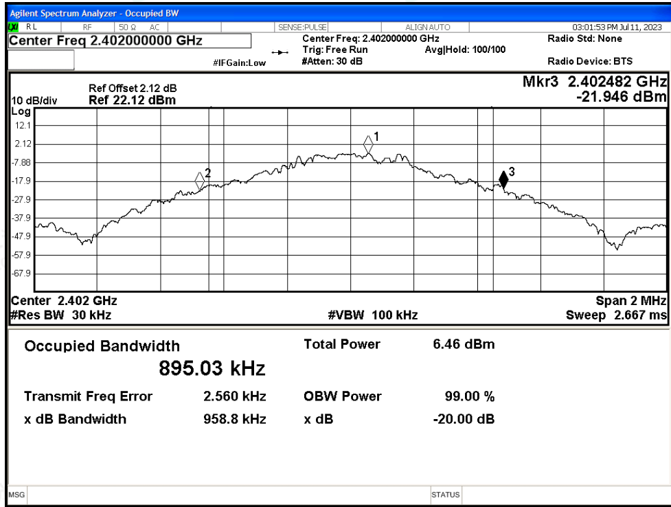
-20dB Bandwidth NVNT 1-DH5 2441MHz Ant
