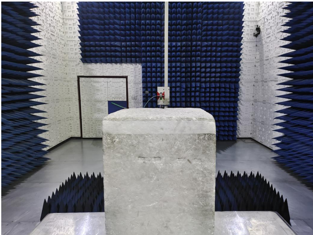
RADIATED EMISSION TEST SETUP ABOVE 1GHz
