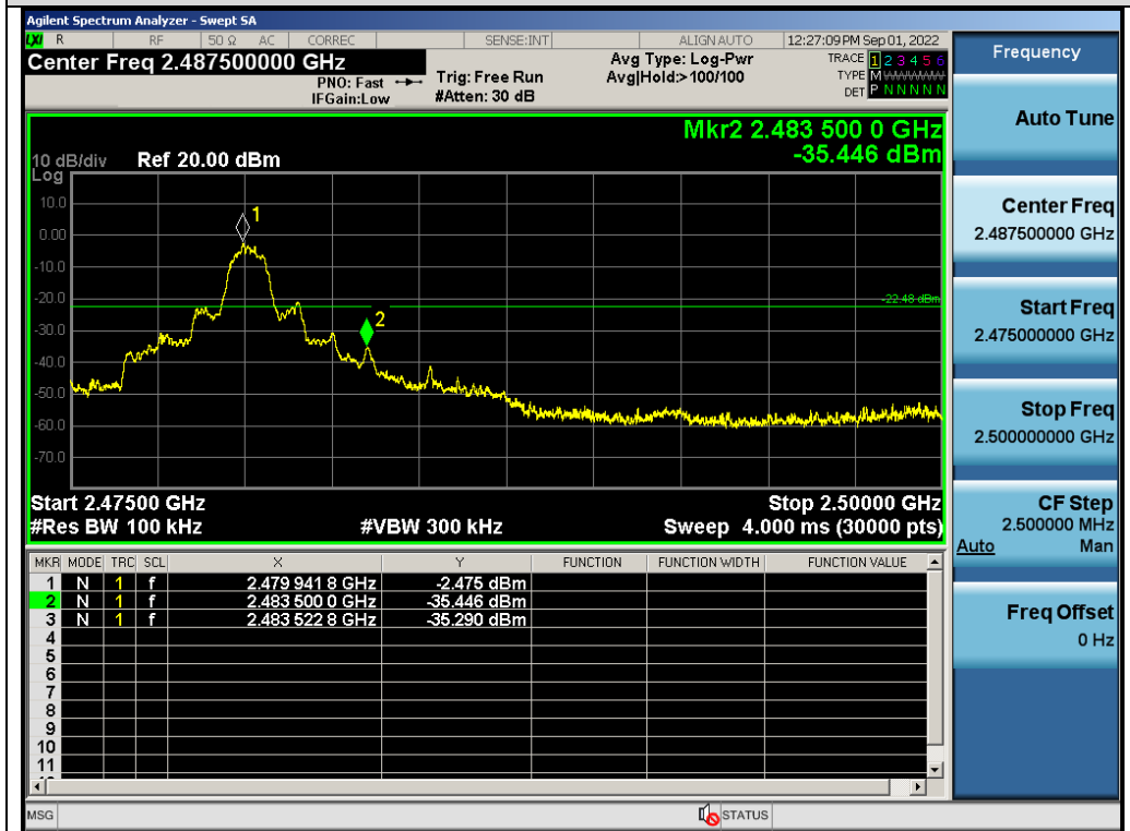
Test_Graph_EDR_ANT1_2480_3Mbps_Higher Band Edge Emissions
