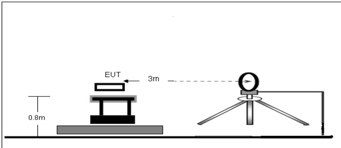
Radiated Emission Test-Up Frequency 30MHz~1GHz
