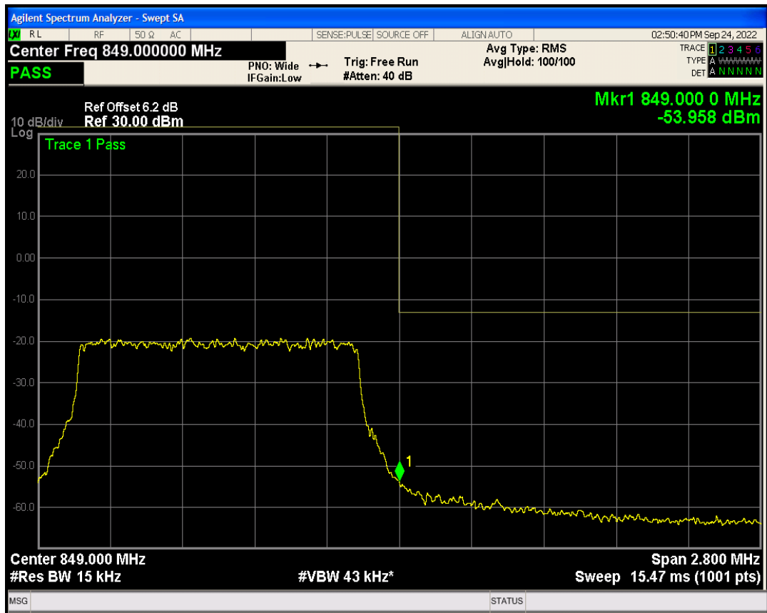
Band5 QPSK BW=3MHz Channel=20415 RB Size=15 Position=#0
