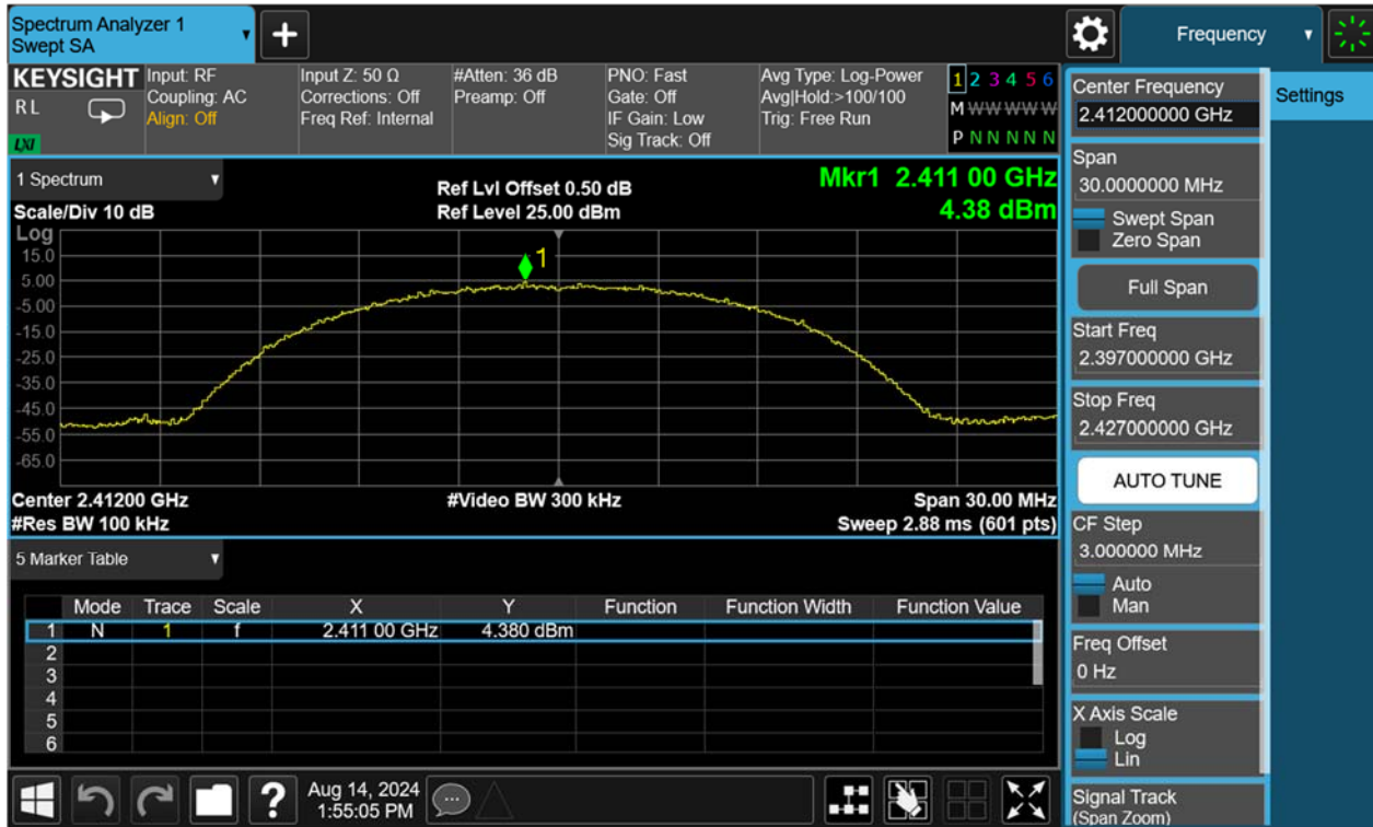
Figure 19: Conducted Spurious Emission & Authorized-band band-edge, 802.11b, 2412MHz Carrier Level
