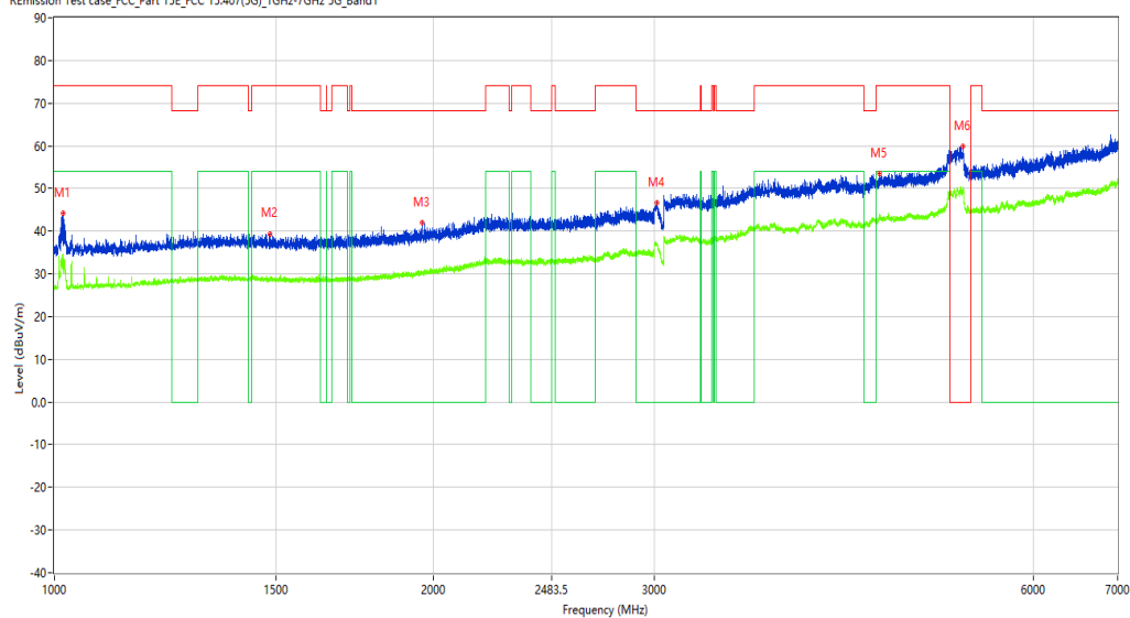
REmission Test case_FCC_Part 15E_FCC 15.407(5G)_1GHz-7GHz_5G_Band1
