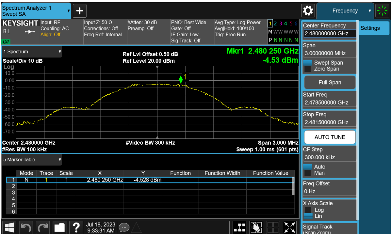
Figure 6: Conducted Spurious Emission & Authorized-band band-edge, 2480MHz, BLE Carrier Level
