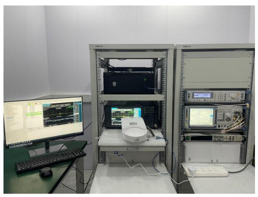
1.3 Set-up for Spurious Emissions below 1GHz
