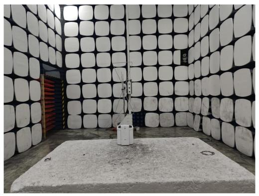
1.4 Set-up for Spurious Emissions above 1GHz
