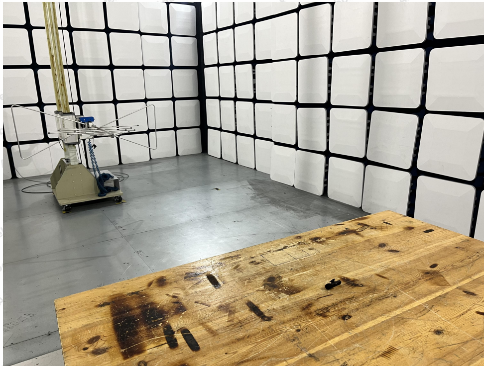
Photo of Radiation Emission Test
