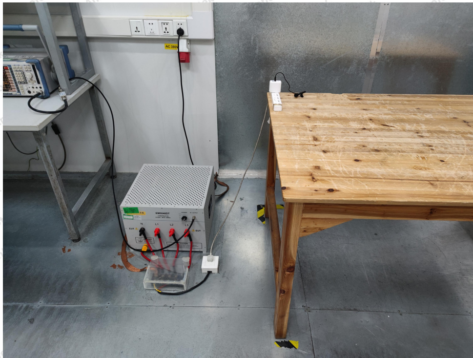
Photo of Conducted Emission Measurement
