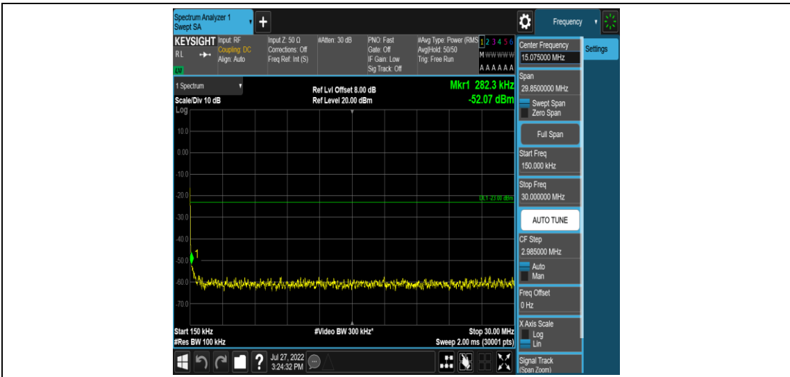
Band12-Stand-Alone-NaN-QPSK-23011-1 @0-3.75kHz-0.15-30-0.15~30MHz@-52.07dBm--2 3-PASS
