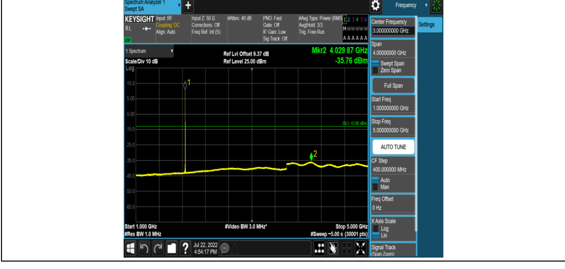
Band2-Stand-Alone-NaN-QPSK-18601-1 @47-3.75kHz-30-1000-30~1000MHz@ -33.72dBm--13-PASS
