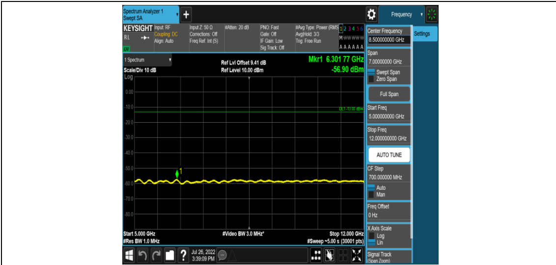
Band2-Stand-Alone-NaN-BPSK-18876-1 @0-15kHz-5000-12000-5000~12000MHz @-56.9dB m--13-PASS
