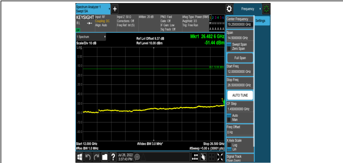
Band2-Stand-Alone-NaN-BPSK-18601-1 @ 11-15kHz-12000-26500-12000~26500MHz@ -51.4 4dBm--13-PASS
