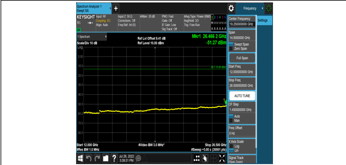
Band2-Stand-Alone-NaN-BPSK-18876-1 @0-15kHz-12000-26500-12000~26500MHz @-51.27 dBm--13-PASS
