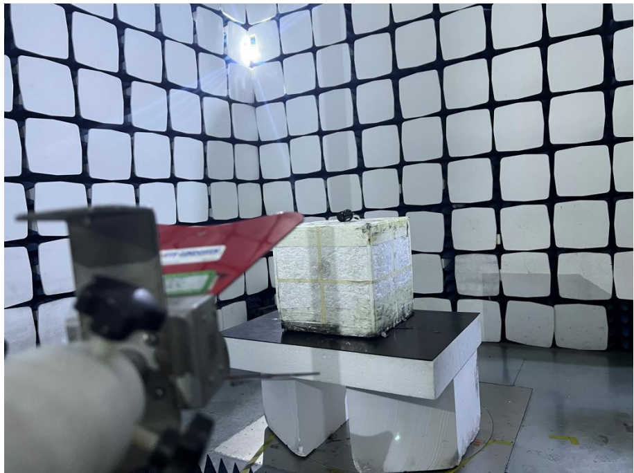
Radiation Emission Test Setup (1GHz to 18GHz)
