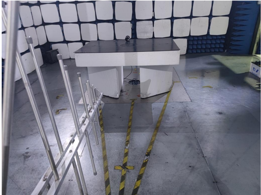
Radiation Emission Test Setup (30MHz to 1GHz)
