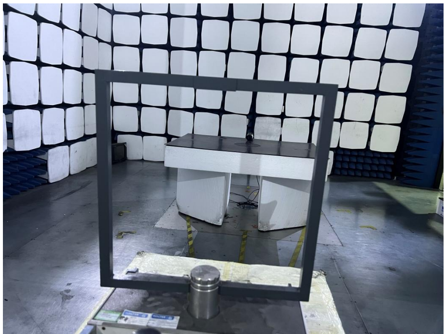
Radiation Emission Test Setup (Below 30MHz)
