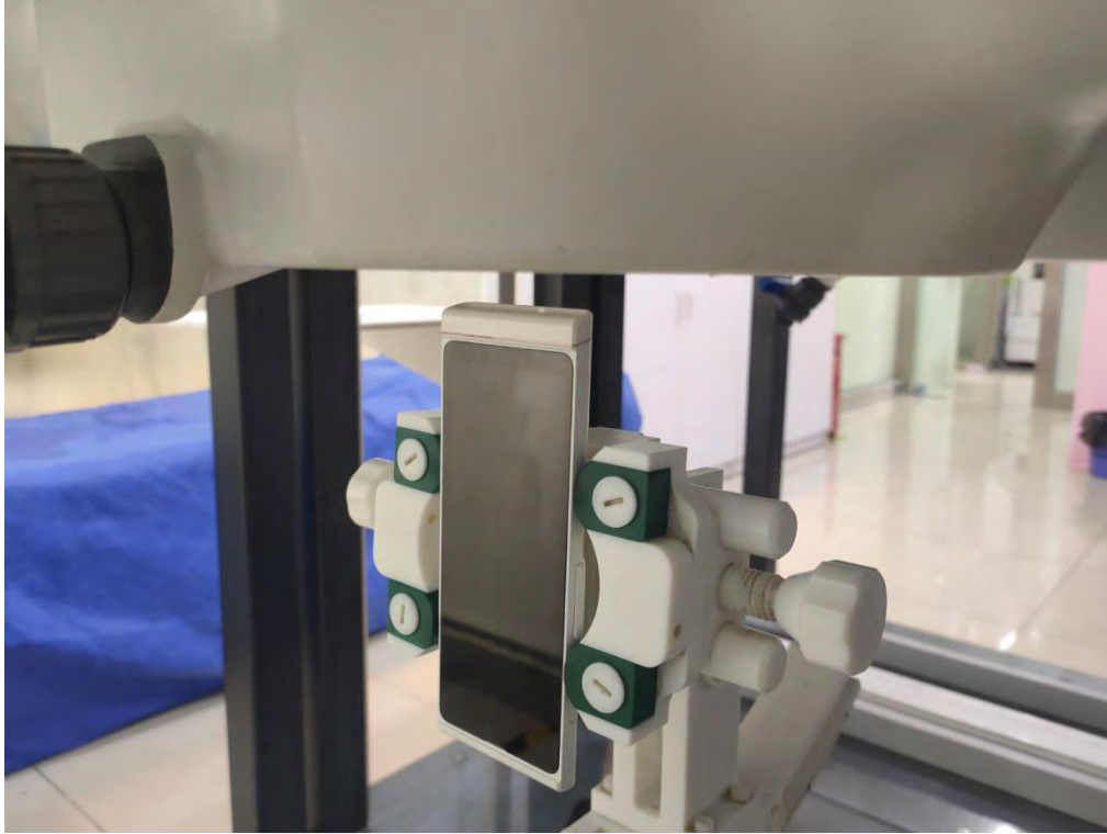
Body Bottom side(separation distance is 10mm)
