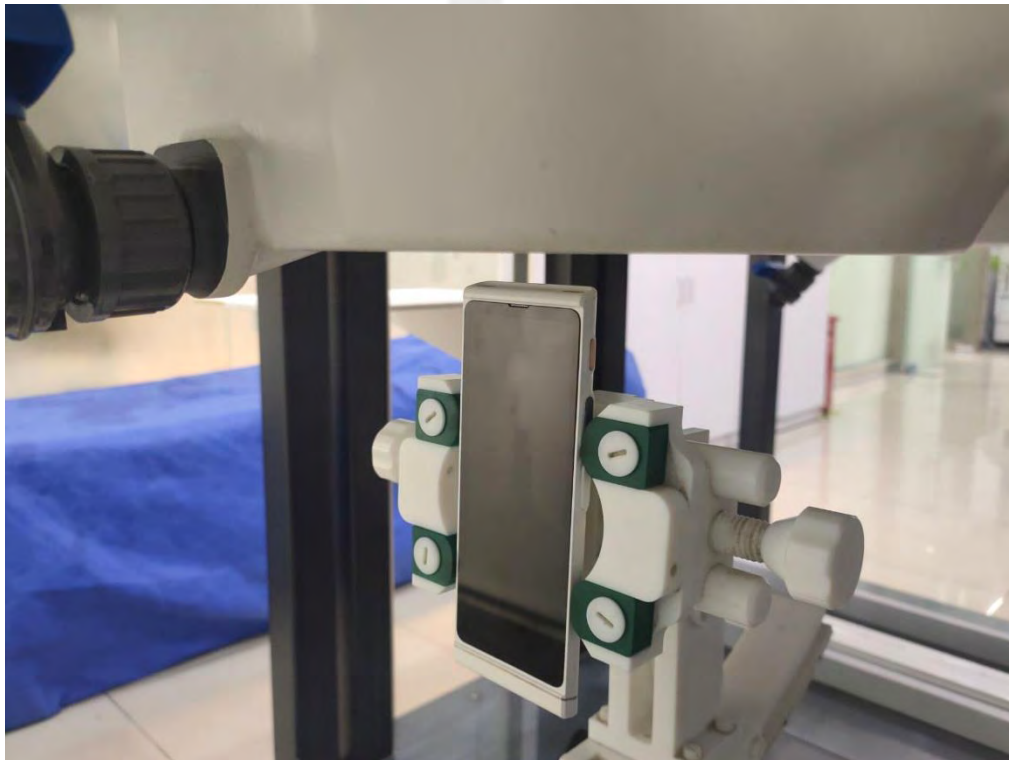
Body Top side(separation distance is 10mm)
