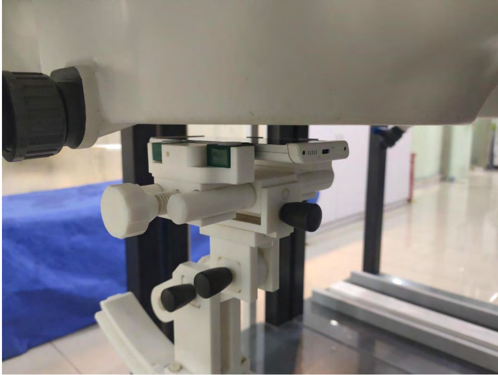
Body Front side(separation distance is 10mm)
