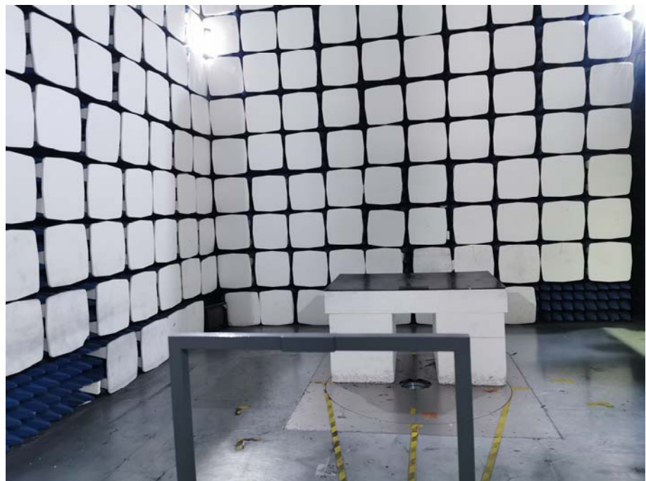
Radiation Emission Test Setup (Below 30MHz)
