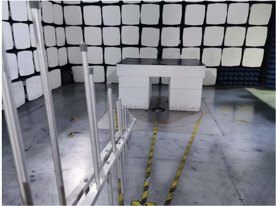
Radiation Emission Test Setup (30MHz to 1GHz)
