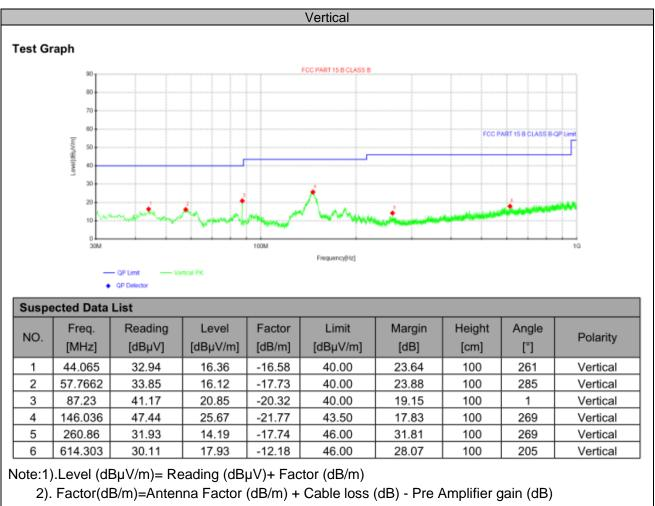
3). Margin(dB) = Limit (dB $\mu$ V/m) - Level (dB $\mu$ V/m)
