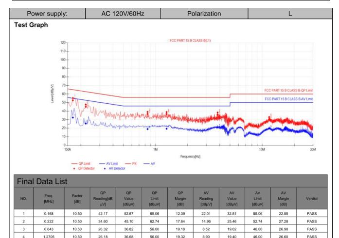
19.90 Note:1).QP Value (dBµV)= QP Reading (dBµV)+ Factor (dB)
