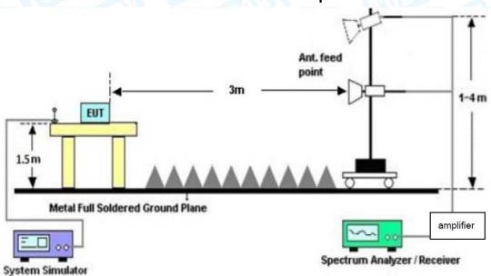
Above 1GHz Test Setup
