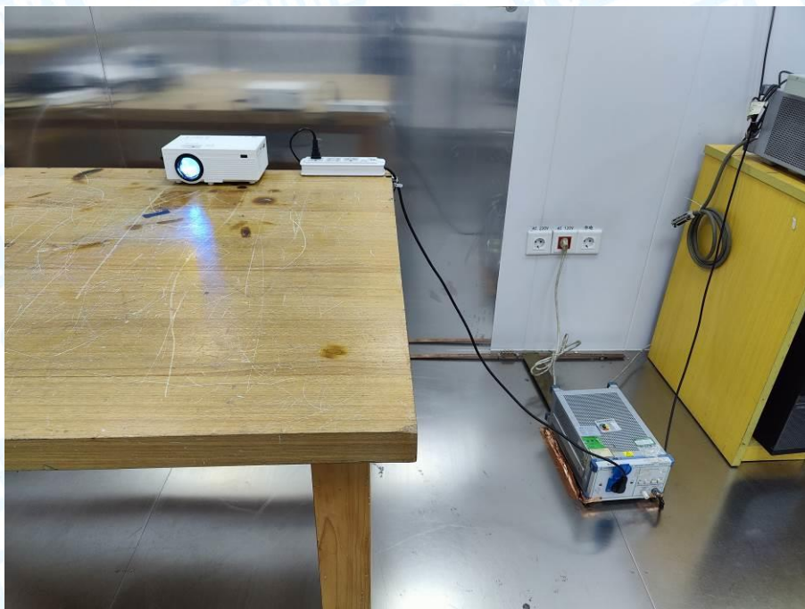
Photo of Setup for Conducted Emission
