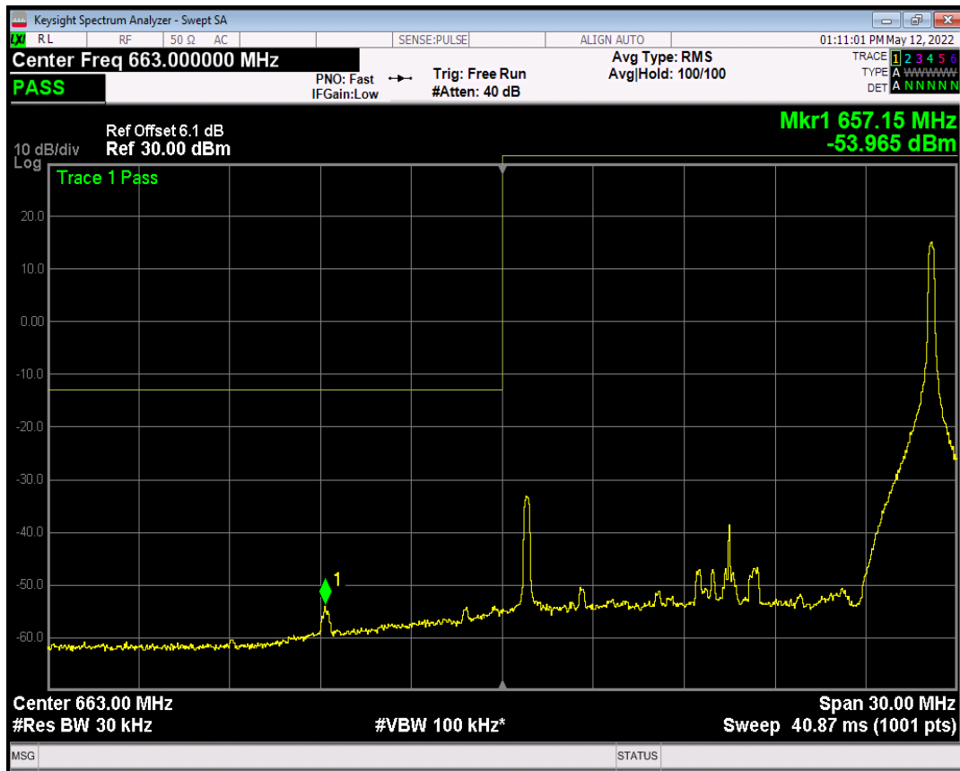
Band71 QPSK BW=15MHz Channel=133197 RB Size=75 Position=#0
