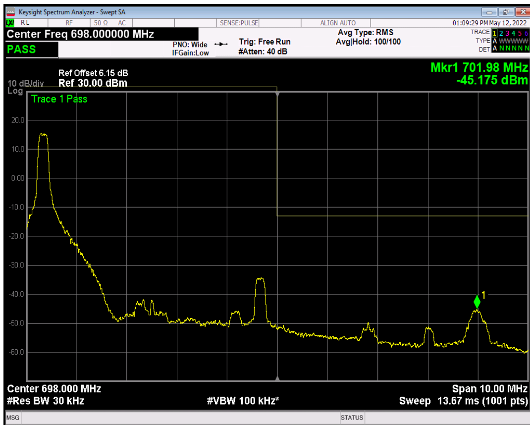
Band71 QPSK BW=5MHz Channel=133447 RB Size=1 Position=#Max
