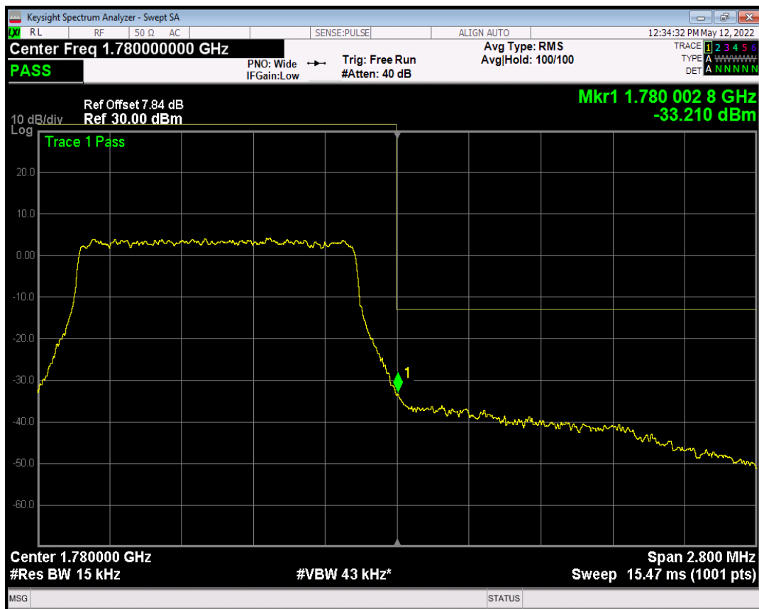
Band66 QAM16 BW=1.4MHz Channel=132665 RB Size=1 Position=#0
