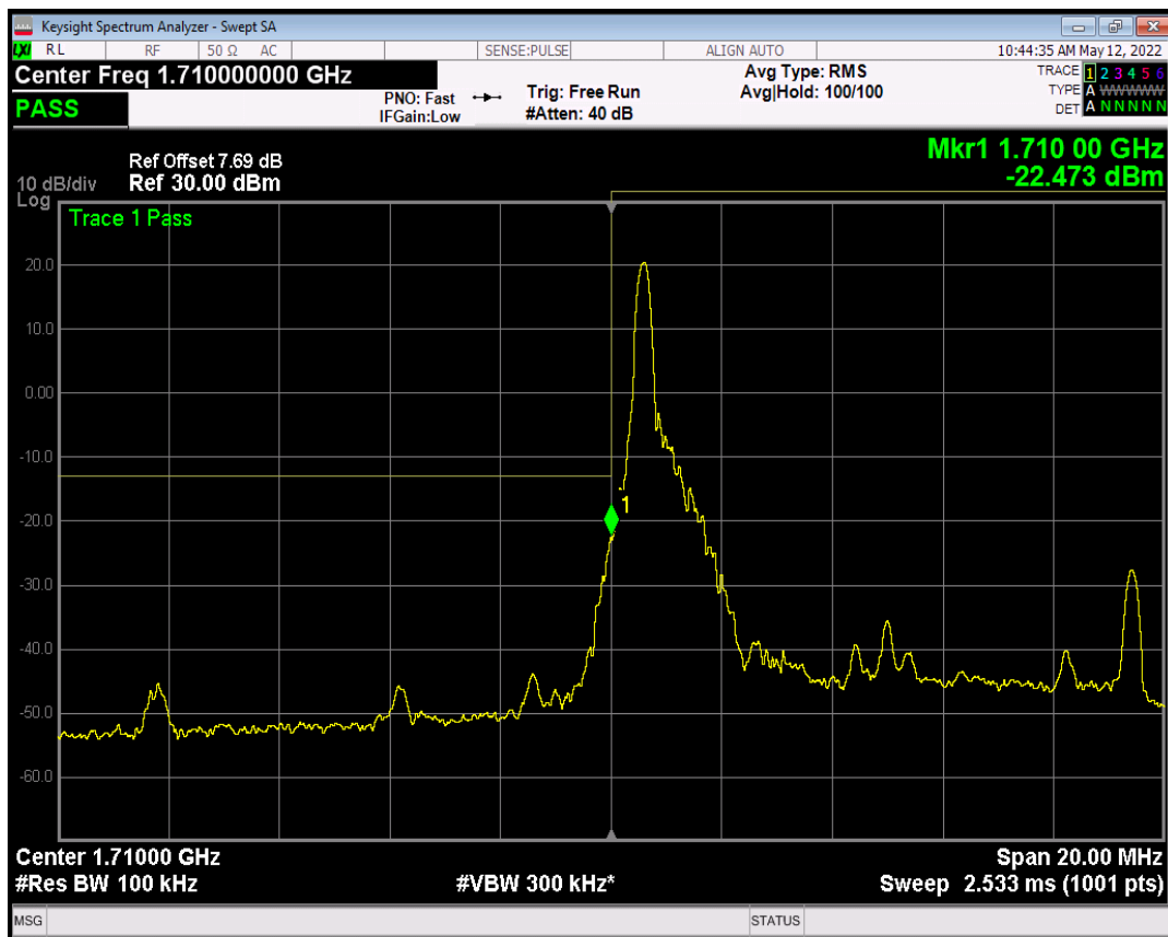
Band4 QPSK BW=10MHz Channel=20000 RB Size=1 Position=#Max
