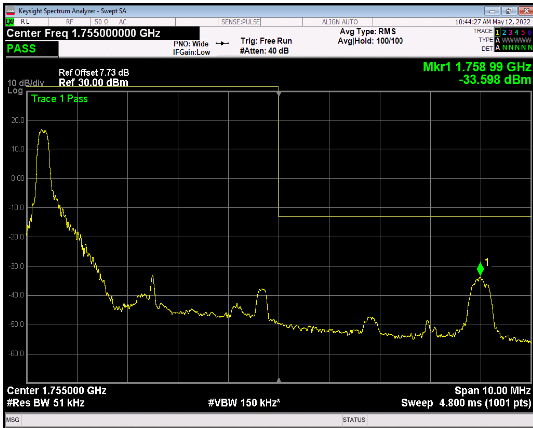
Band4 QAM16 BW=5MHz Channel=20375 RB Size=1 Position=#Max
