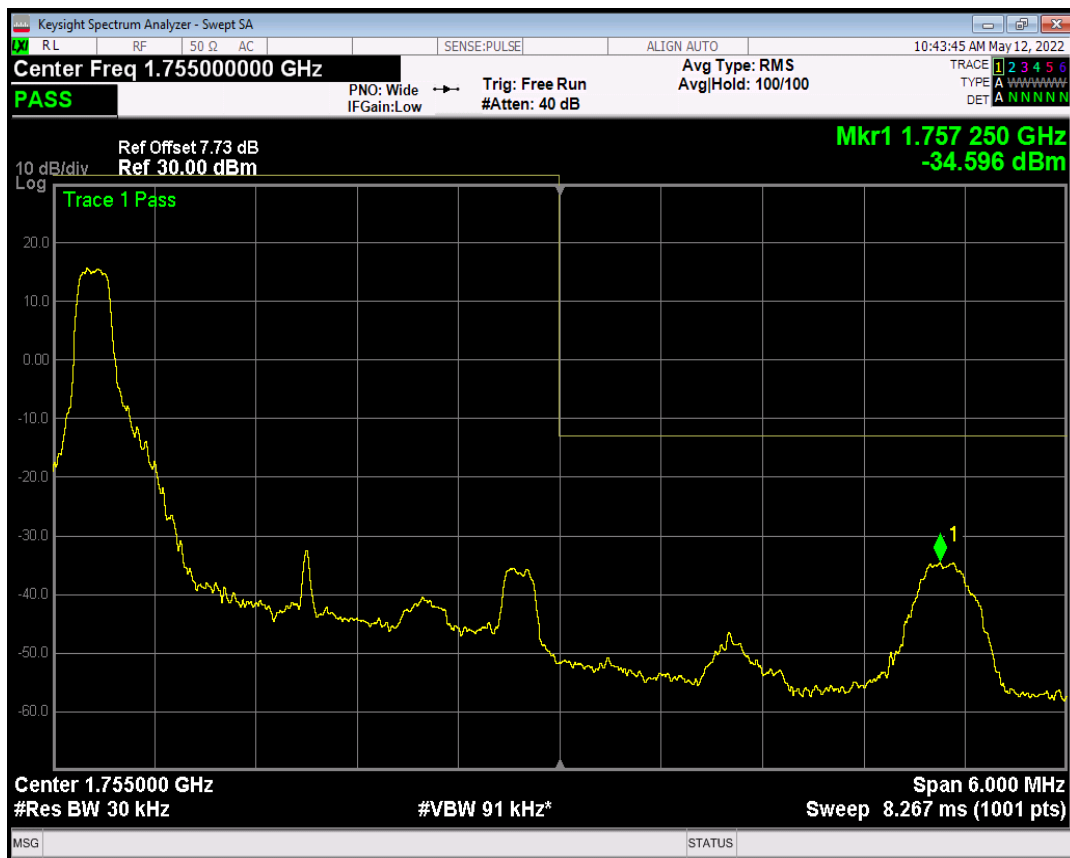
Band4 QPSK BW=3MHz Channel=20385 RB Size=1 Position=#Max
