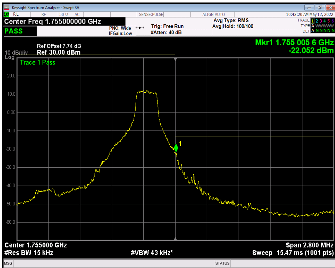
Band4 QAM16 BW=1.4MHz Channel=20393 RB Size=6 Position=#0
