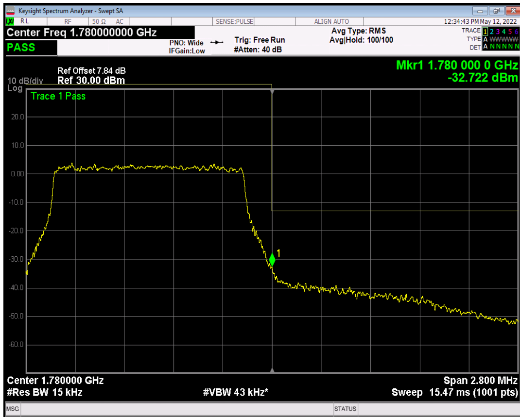
Band66 QPSK BW=3MHz Channel=131987 RB Size=1 Position=#0
