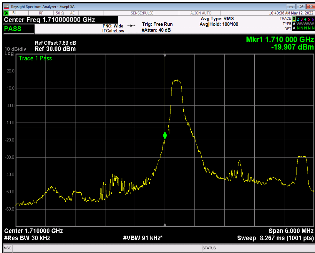
Band4 QAM16 BW=3MHz Channel=19965 RB Size=1 Position=#Max
