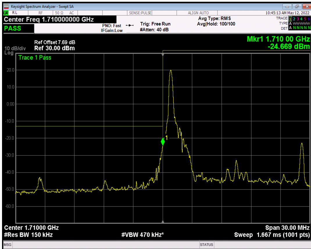
Band4 QAM16 BW=15MHz Channel=20025 RB Size=1 Position=#Max
