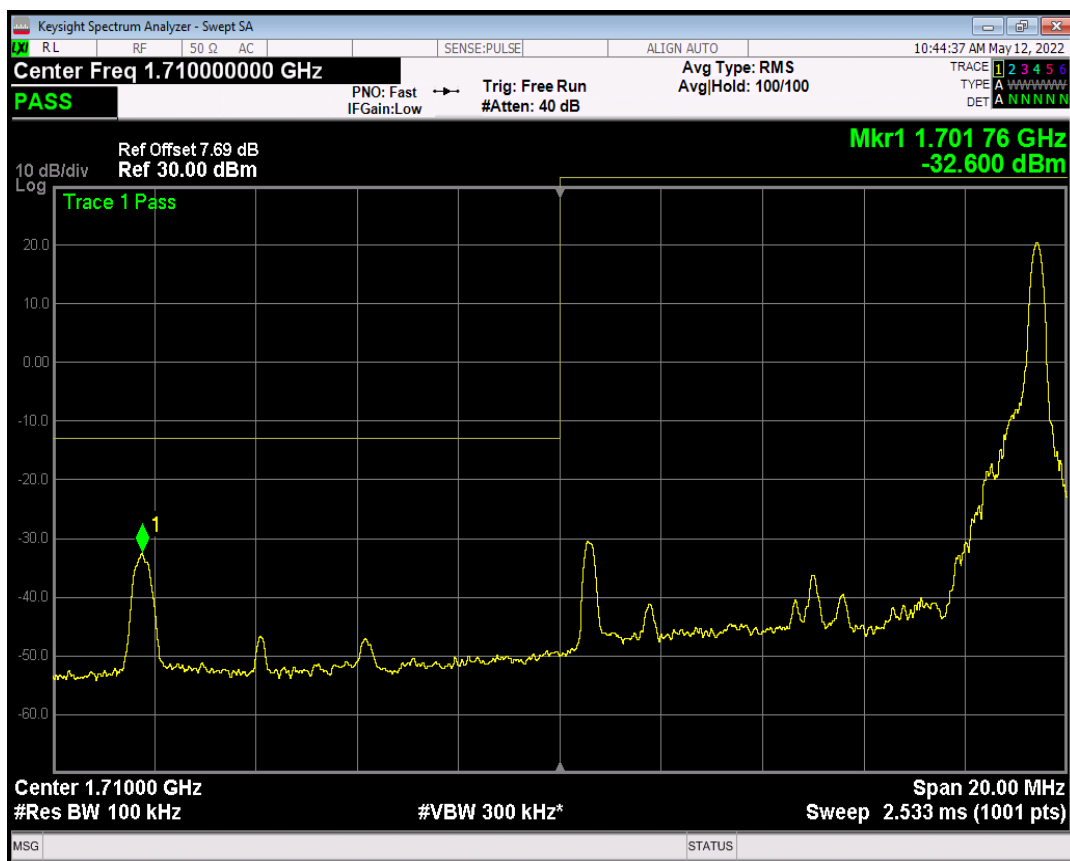
Band4 QPSK BW=10MHz Channel=20000 RB Size=50 Position=#0
