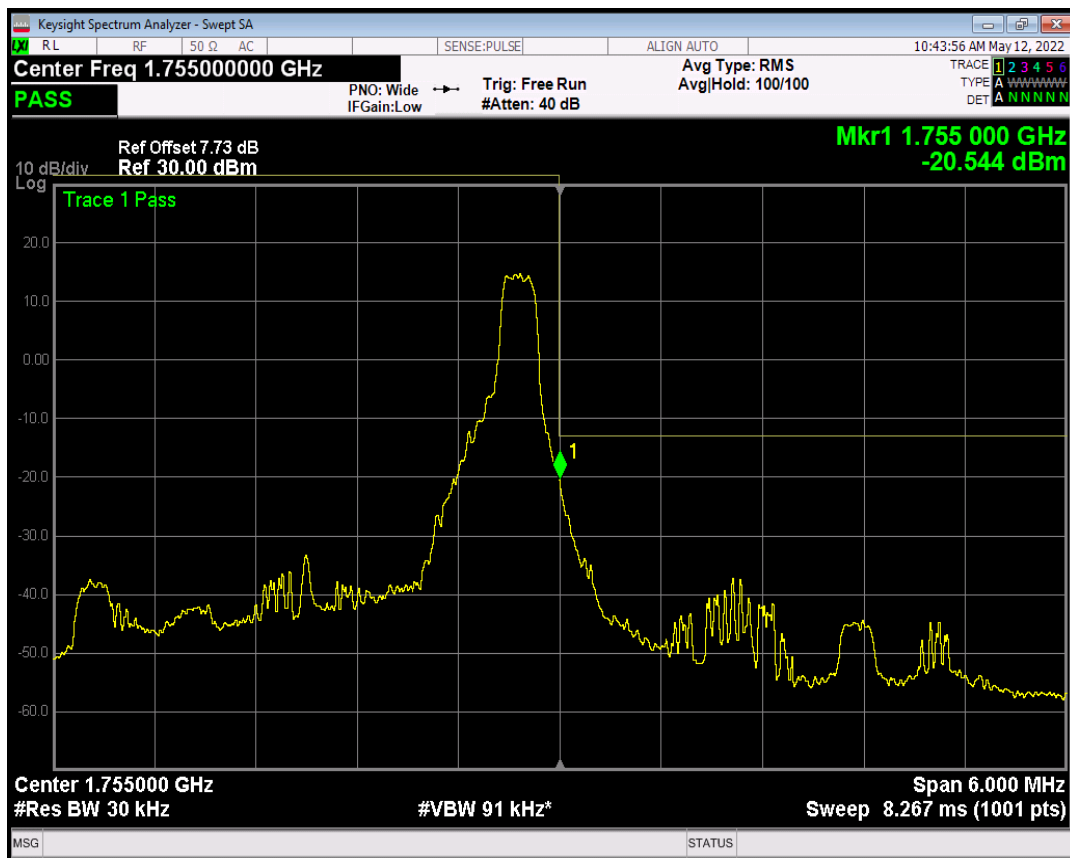
Band4 QAM16 BW=3MHz Channel=20385 RB Size=15 Position=#0
