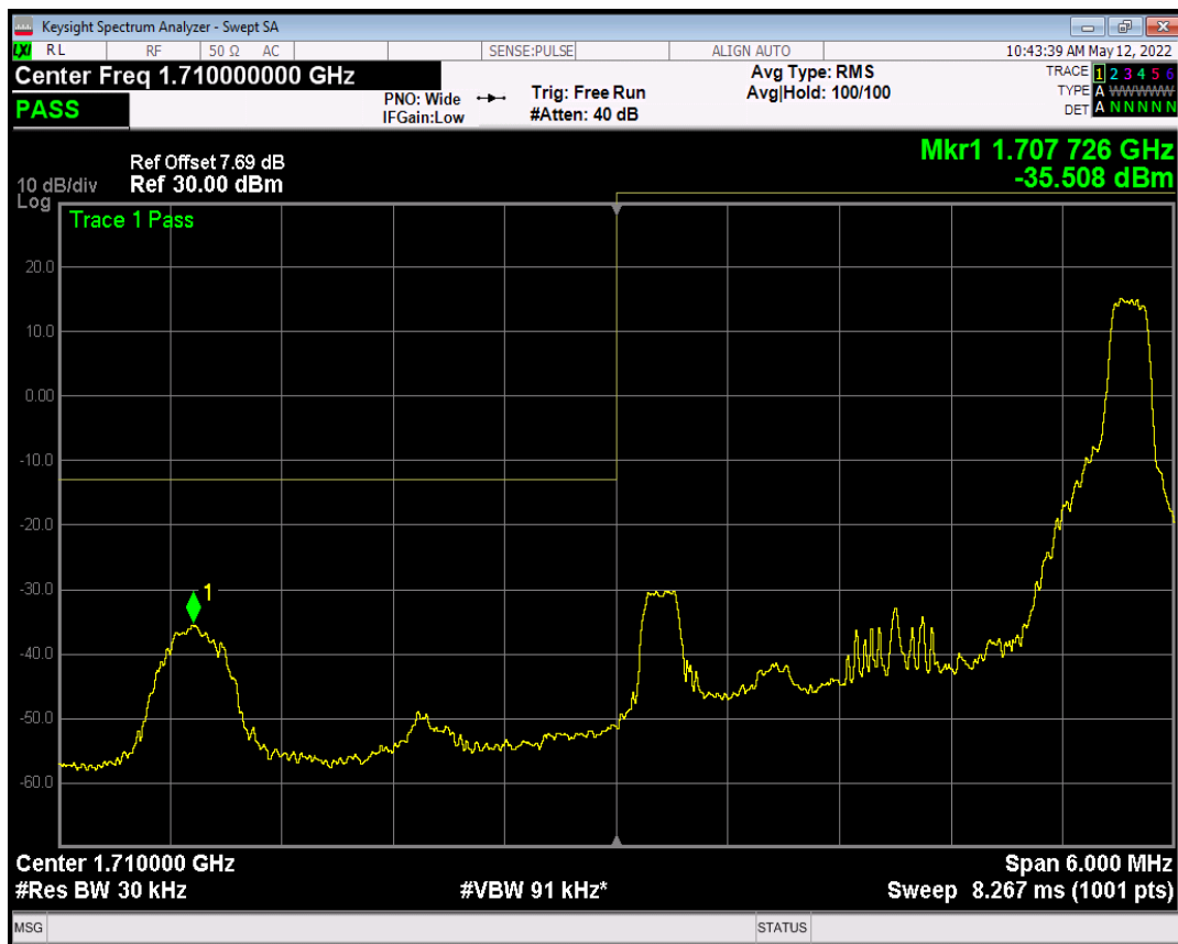
Band4 QAM16 BW=3MHz Channel=19965 RB Size=15 Position=#0
