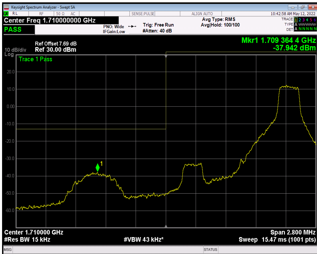
Band4 QAM16 BW=1.4MHz Channel=19957 RB Size=6 Position=#0
