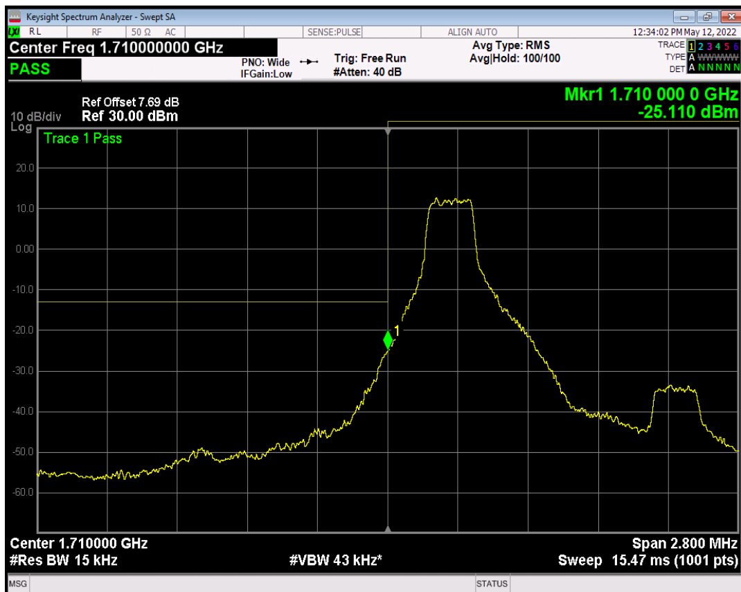
Band66 QPSK BW=1.4MHz Channel=131979 RB Size=1 Position=#Max
