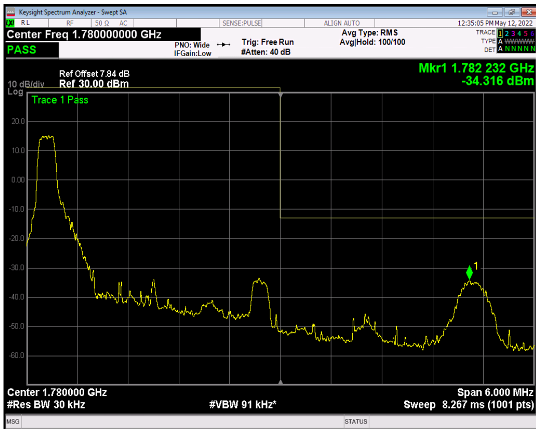
Band66 QPSK BW=3MHz Channel=132657 RB Size=1 Position=#Max
