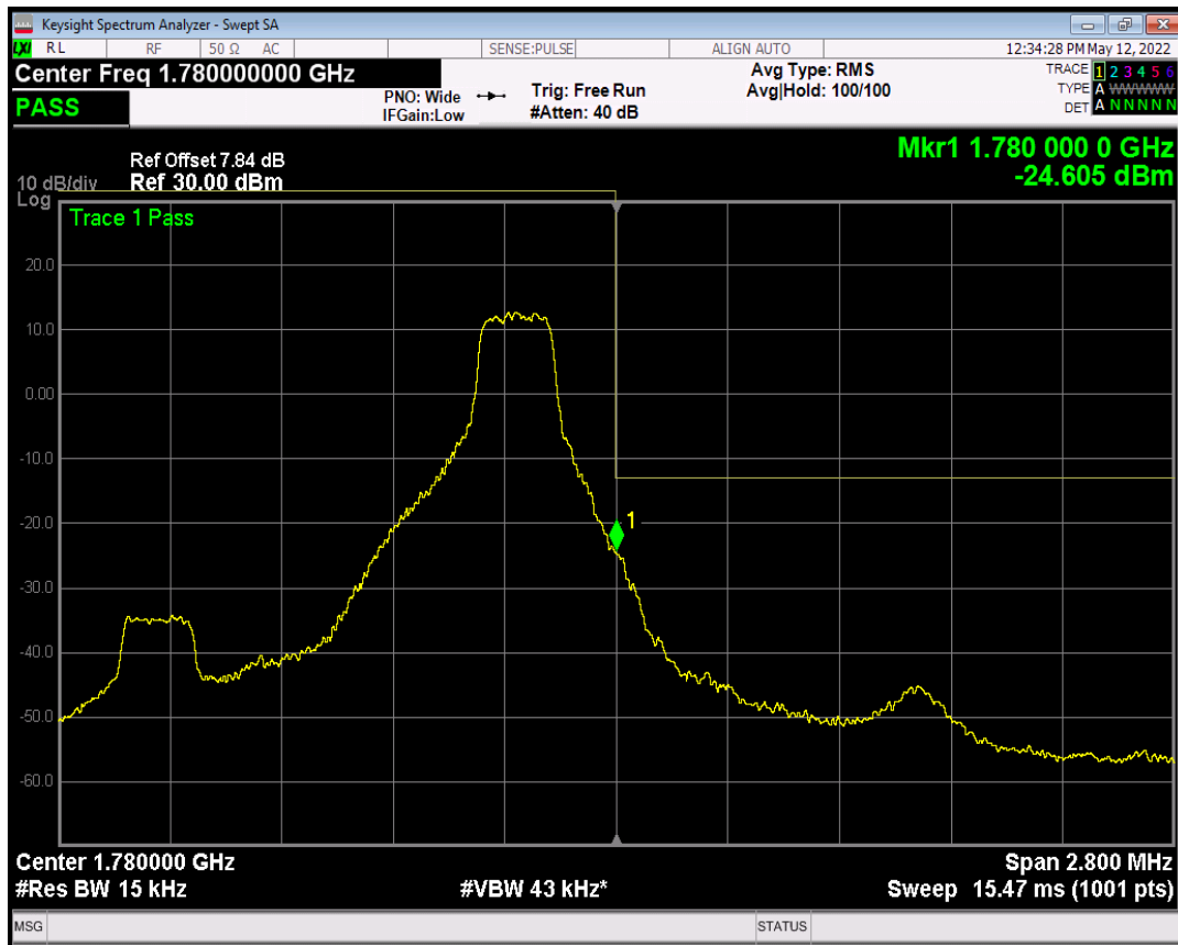
Band66 QPSK BW=1.4MHz Channel=132665 RB Size=6 Position=#0
