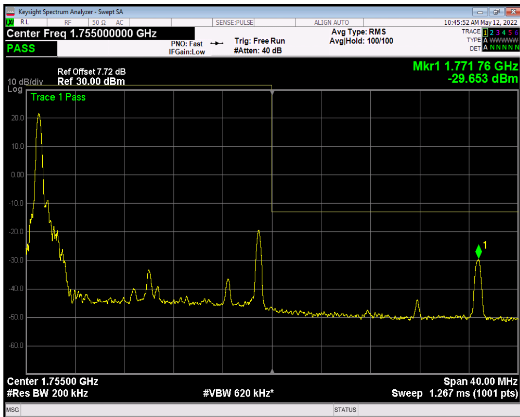
Band4 QPSK BW=20MHz Channel=20300 RB Size=1 Position=#Max
