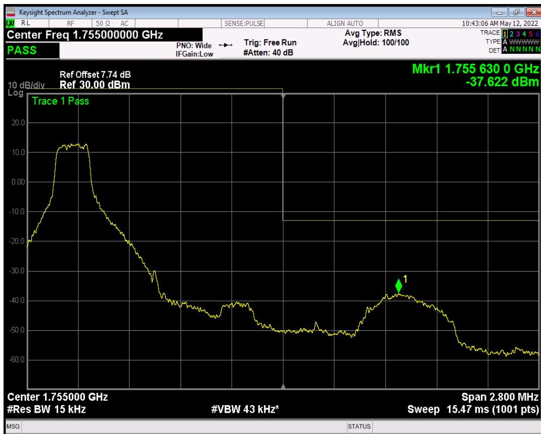
Band4 QPSK BW=1.4MHz Channel=20393 RB Size=1 Position=#Max
