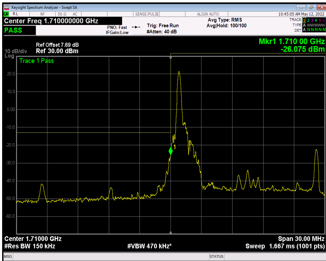
Band4 QPSK BW=15MHz Channel=20025 RB Size=1 Position=#Max
