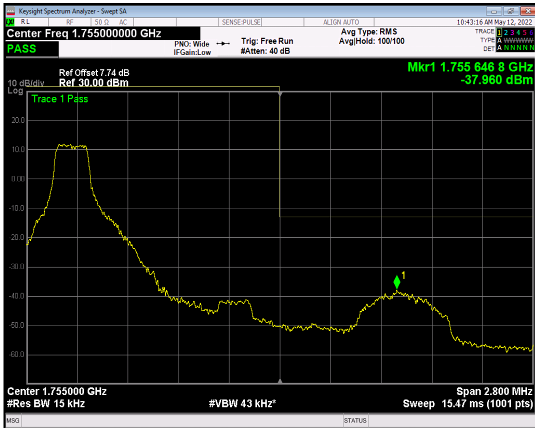
Band4 QAM16 BW=1.4MHz Channel=20393 RB Size=1 Position=#Max
