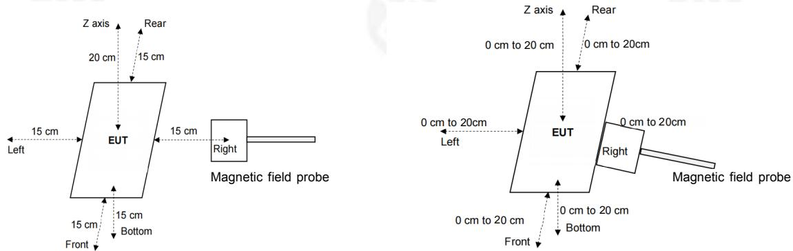
Note: Measurements should be made from all sides and the top of the primary/client pair, with the 20 cm-0cm measured from the center of the top, and 20cm-0cm measured from the center of the rest
