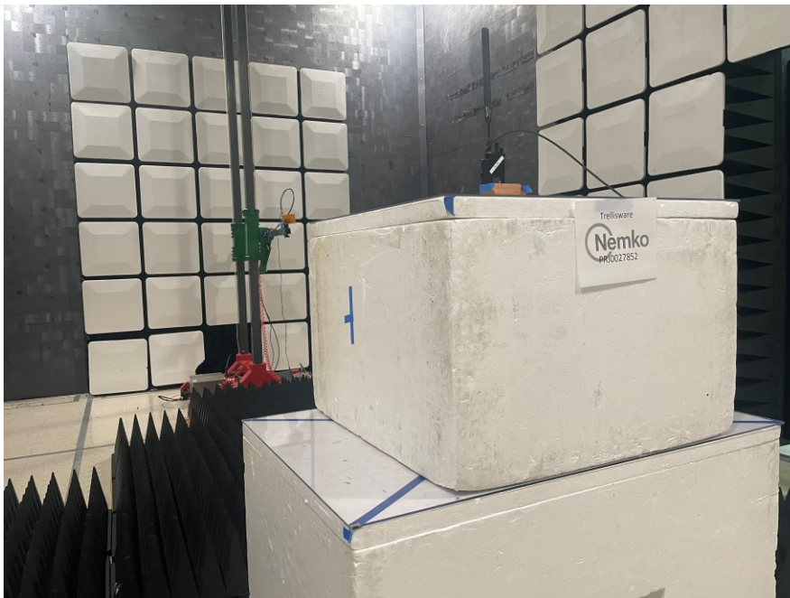
Figure 7 - Radiated emissions above 1 GHz (18 – 26.5 GHz)
