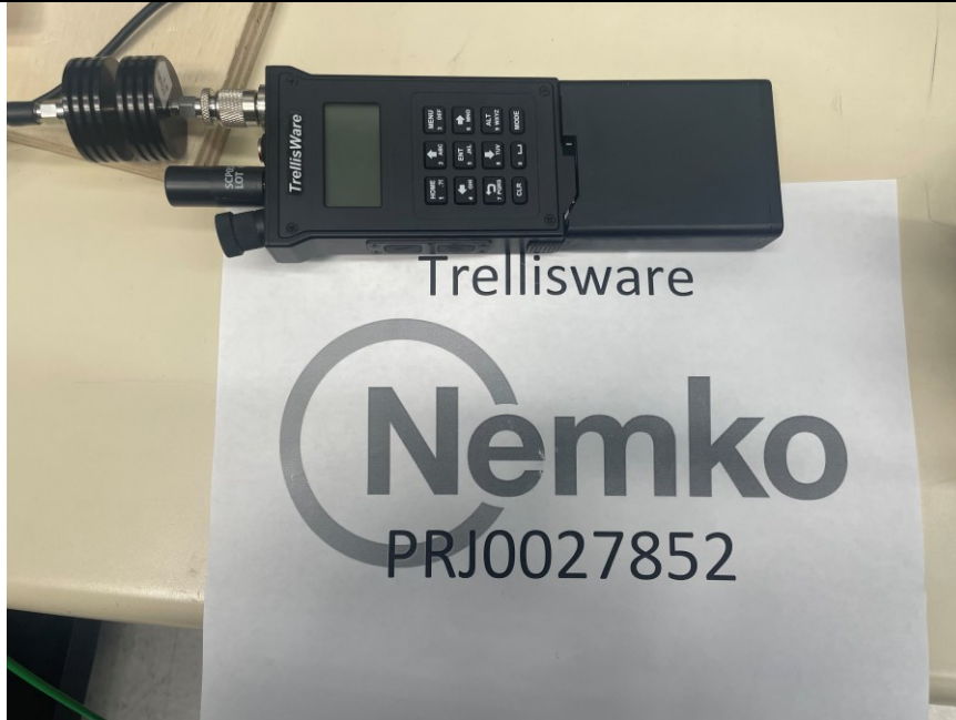
Figure 10 – Test setup, antenna conducted port.
