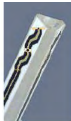
Figure 2.3 Probe Thick-Film Technique
