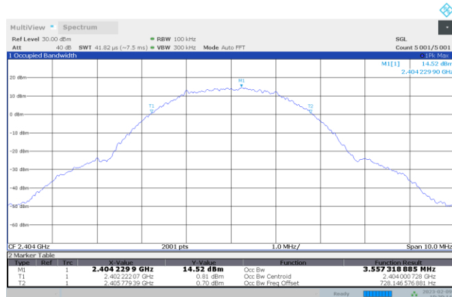
Figure 8.6-4: TSM-Bandwidth 3.6MHz 99 % occupied bandwidth, 2404 MHz
