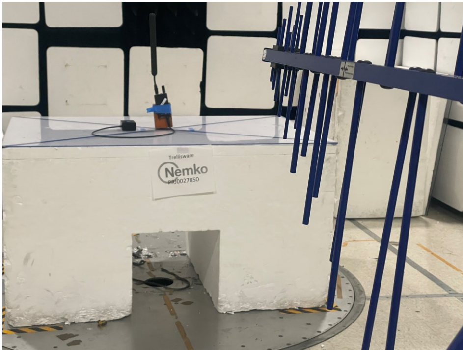
Figure 2 - Radiated emissions below 1 GHz (0.03 – 1 GHz), front view.
