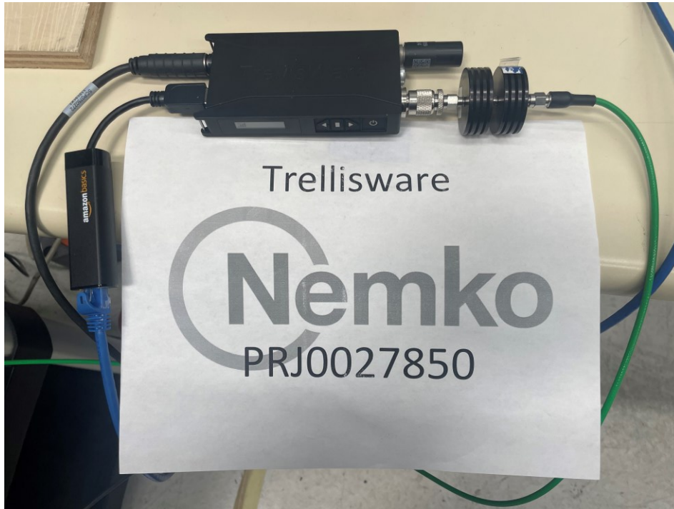
Figure 10 – Test setup, antenna conducted port.
