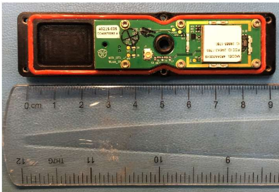
Figure 6: TW-1760 PCB, shield-can removed
