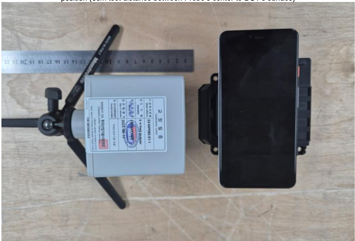
position (6cm test distance between Probe's center to DUT's surface)
