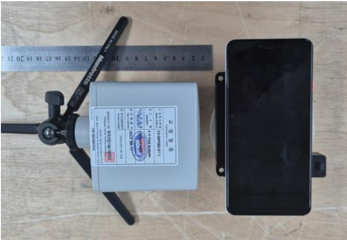
Right position (6cm test distance between Probe's center to DUT's surface)
