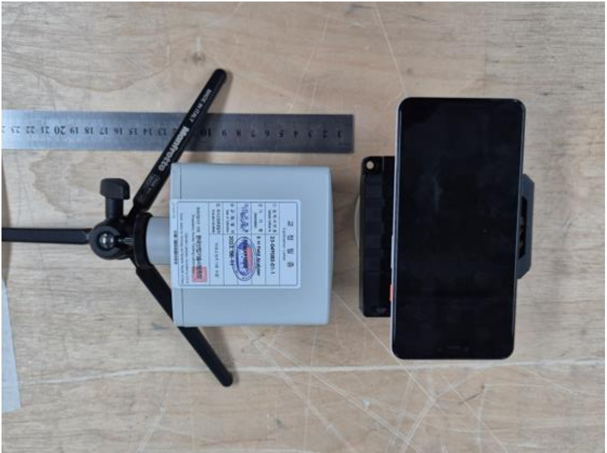
position (6cm test distance between Probe's center to DUT's surface)
