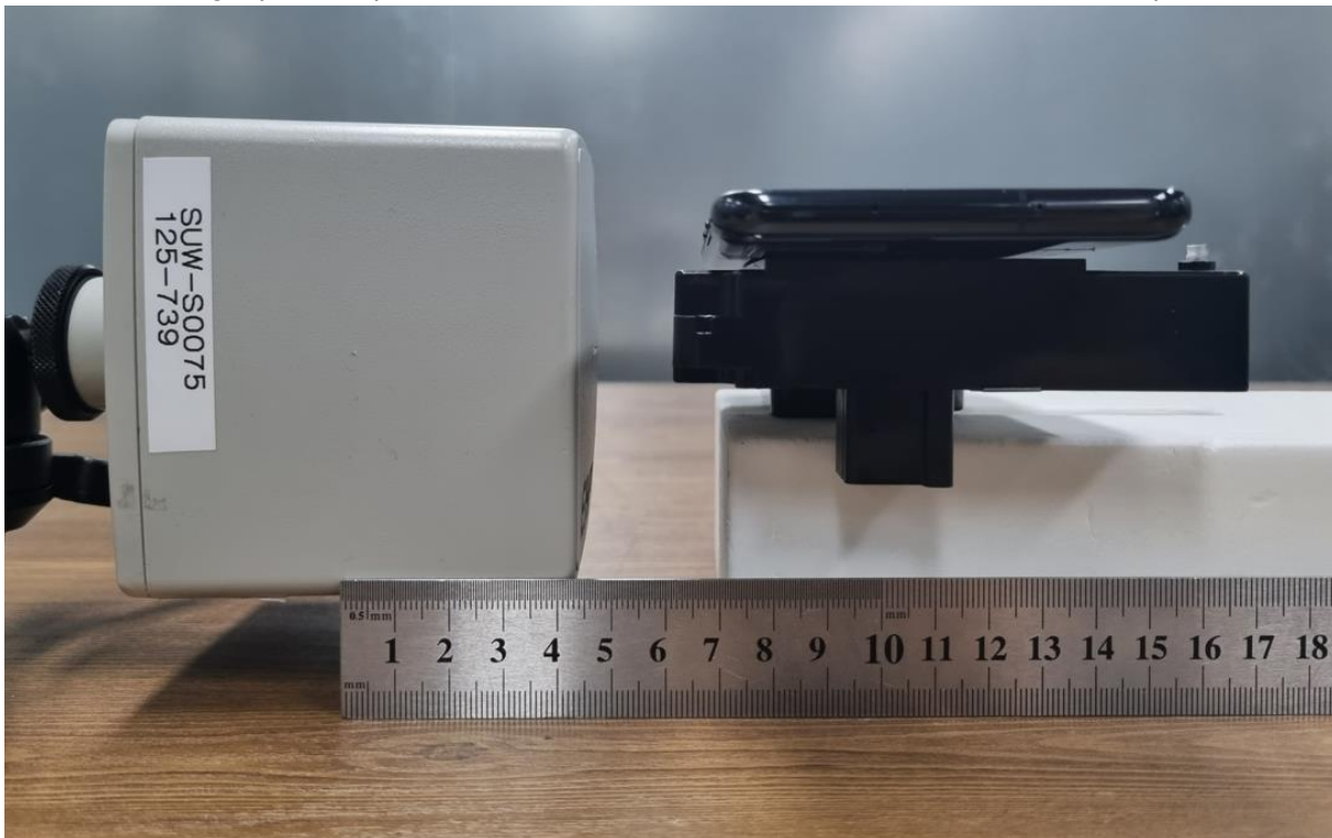
Right position (6cm test distance between Probe's center to DUT's surface)
