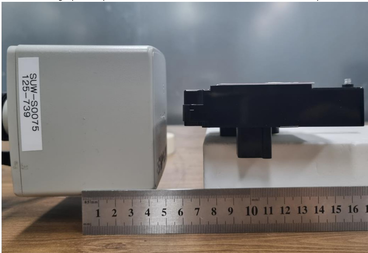
Right position (6cm test distance between Probe's center to DUT's surface)
