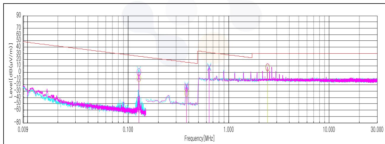
**Middle****Radiated Emissions Fundamental & 9 kHz to 30 MHz**
