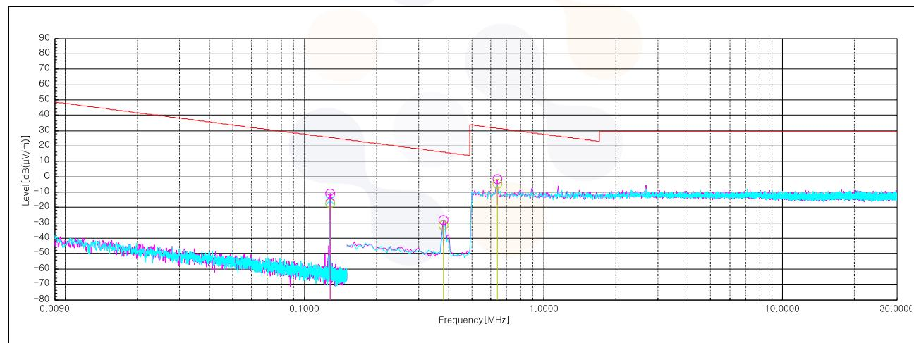
**Right****Radiated Emissions Fundamental & 9 kHz to 30 MHz**
