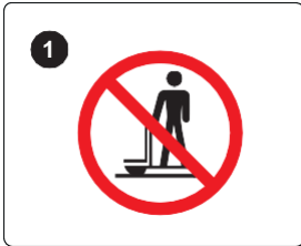
1 Warning sign: Lifting of persons with the forks is prohibited
