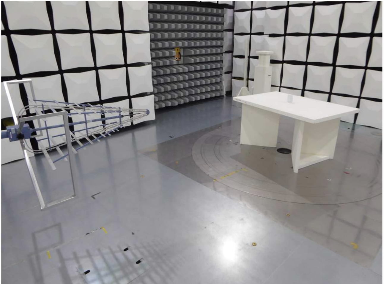
Test setup semi anechoic chamber Table setup (Pos 1)
