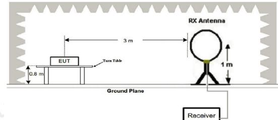
2. Radiated Emission Test-Up Frequency 30MHz~1GHz
