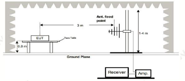
3. Radiated Emission Test-Up Frequency Above 1GHz
