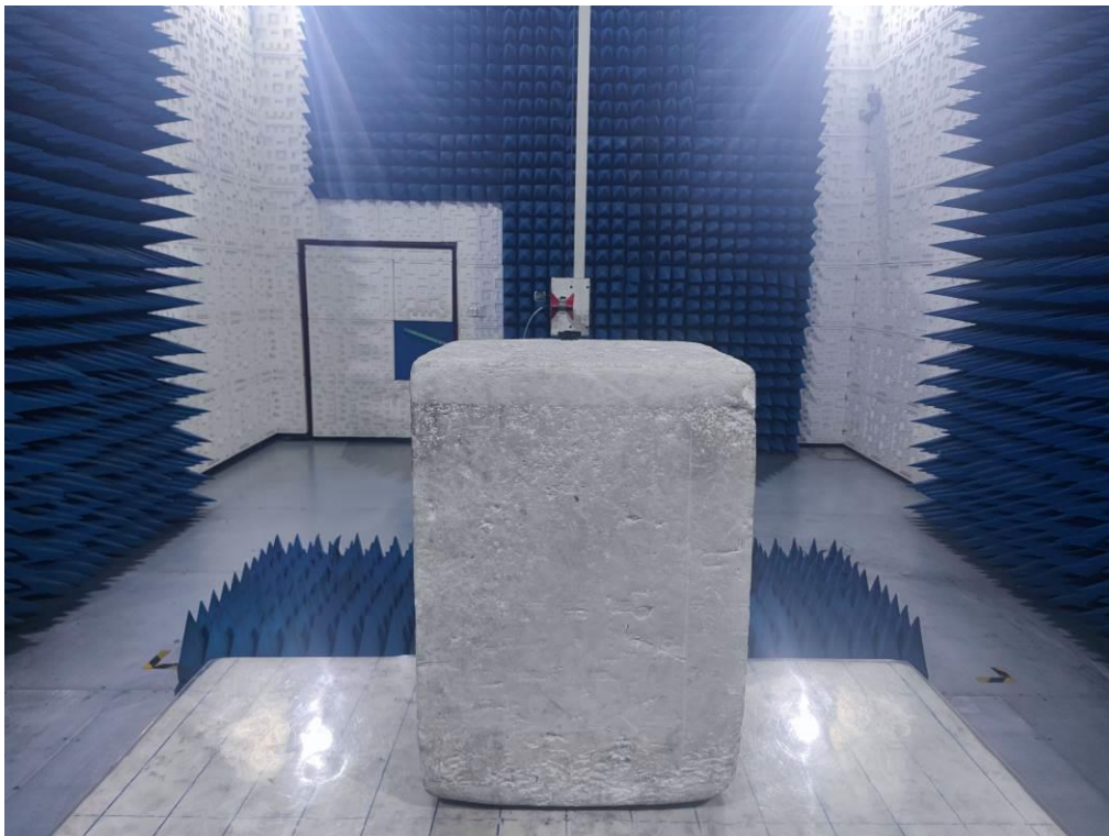
RADIATED EMISSION TEST SETUP ABOVE 1GHz
