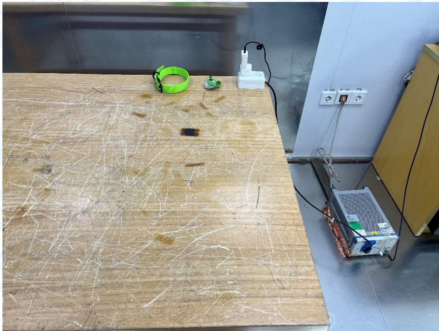
Photo of Setup for Conducted Emission
