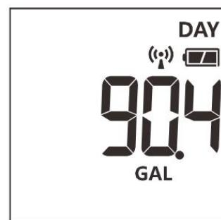
The screen shows the total water consumption each day starting at 0:00. The LCD displays the "DAY," and the unit is either L or GAL with a maximum display value of 999999L or 999999GAL.
