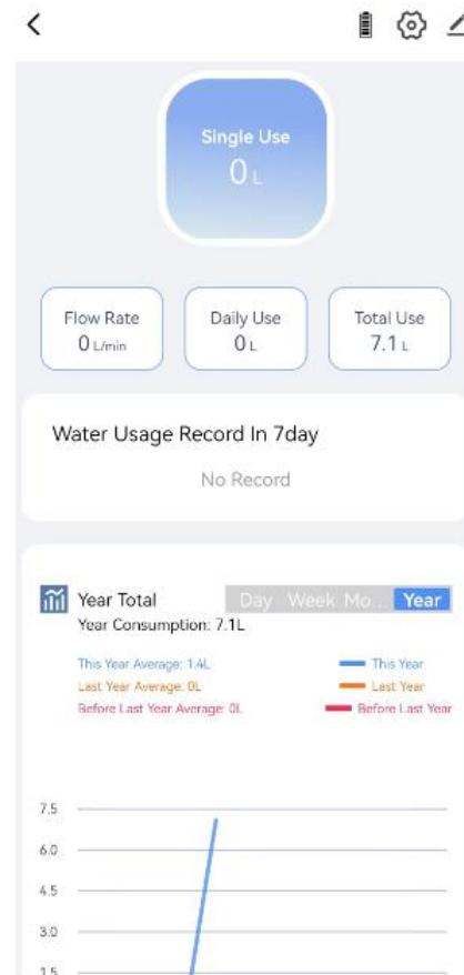
**5.3** On the app, you can view the water usage records for single-use, total water consumption in 24 hours, total water consumed within 1 year, and monthly water consumption for up to 3 years. It can save up to 100 records if the device is disconnected and automatically clears the earliest records when the data exceeds 100.
