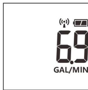
The screen displays the current flow rate value every second in units of L/Min or GAL/Min. The display does not show the leading zero; the maximum value indicated is 41.9L/Min or 11.0GAL/Min. If the flow rate exceeds this value, it will be displayed as HH.H L/Min or HH.H GAL/Min.
