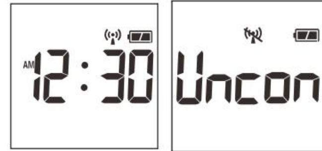
When the LCD is in the off state, press the button to show the current time and connection graph if the product is connected to the smartphone. If disconnected, it will show the disconnection graph. For a paired but disconnected device, it will display "----." When the product is unpaired, it will show "Uncon." Pressing the button again will switch to mode 1.
