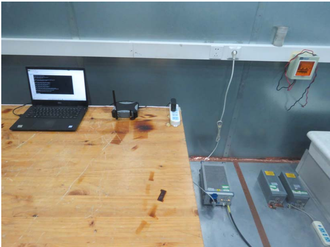
Picture 2 Conducted Emission Test Setup
