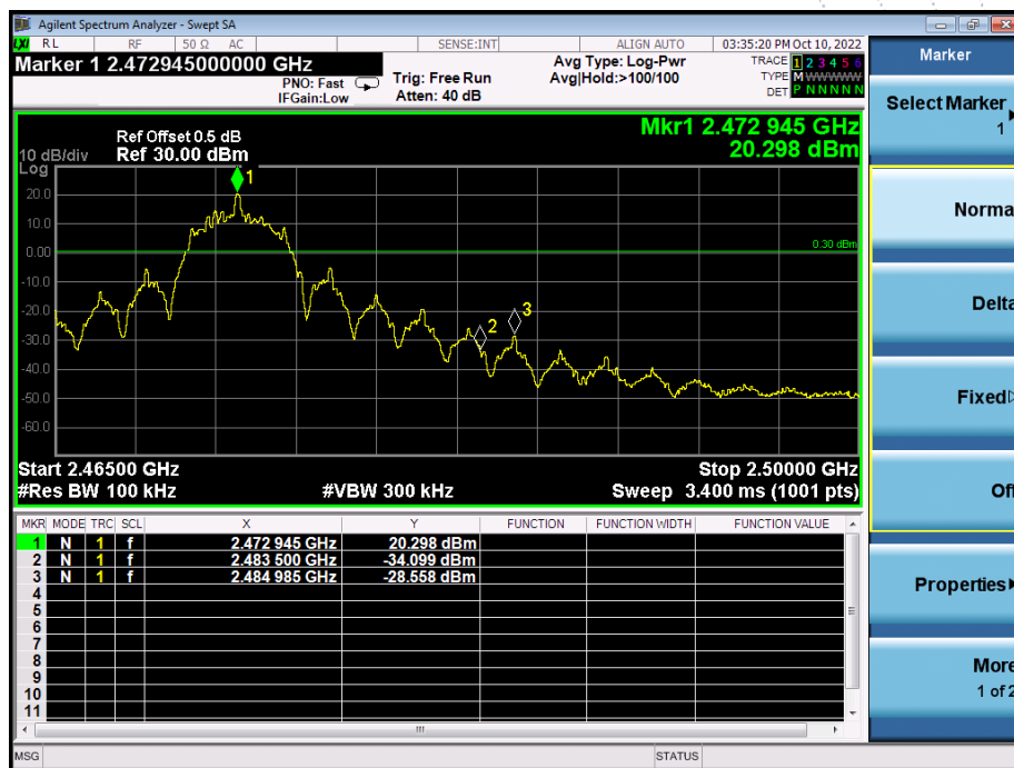
GFSK: Band Edge, Right Side
