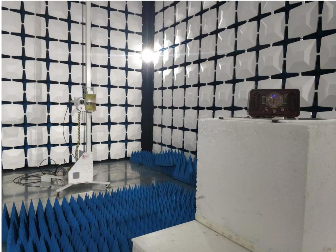
Above 1GHz for radiated emission test setup
