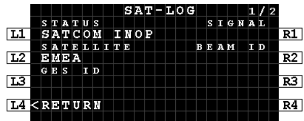
Figure 5-24: TCP - SAT LOG 1/2 - Status - SATCOM INOP
