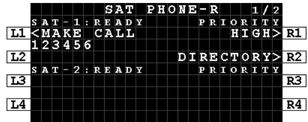
Figure 7-19: TCP - SAT PHONE-R - Manual Entry - Short Code - Pre-selected
