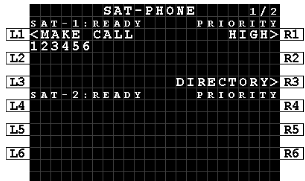
Figure 7-2: MCDU - SAT-PHONE - Manual Entry - Short Code - Pre-selected
