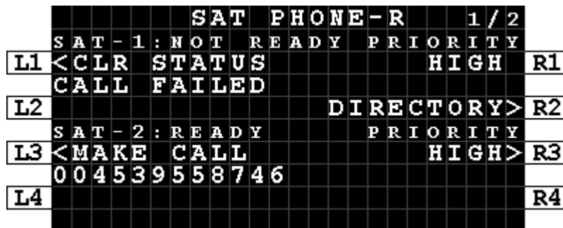
Figure 7-26: TCP - SAT PHONE-R 1/2 - Outgoing Call - Call Failed
