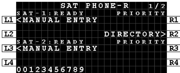
Figure 7-18: TCP - SAT PHONE-R 1/2 - Manual Entry - International Number - Scratchpad
