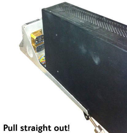
Figure 7-5: Pull out the LRU
