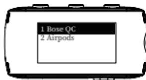
④ Press the menu up/down buttons to select Bluetooth device, and press the confirm button to select and pair
