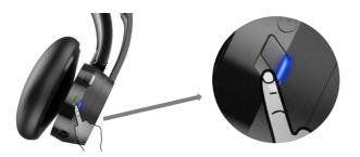
Step 1: Push the power button up to the top, press and hold for 3 seconds, then release. The blue light flashes for 3 seconds, then the red and blue lights flash alternately. You will hear the "Pairing" voice prompt.
