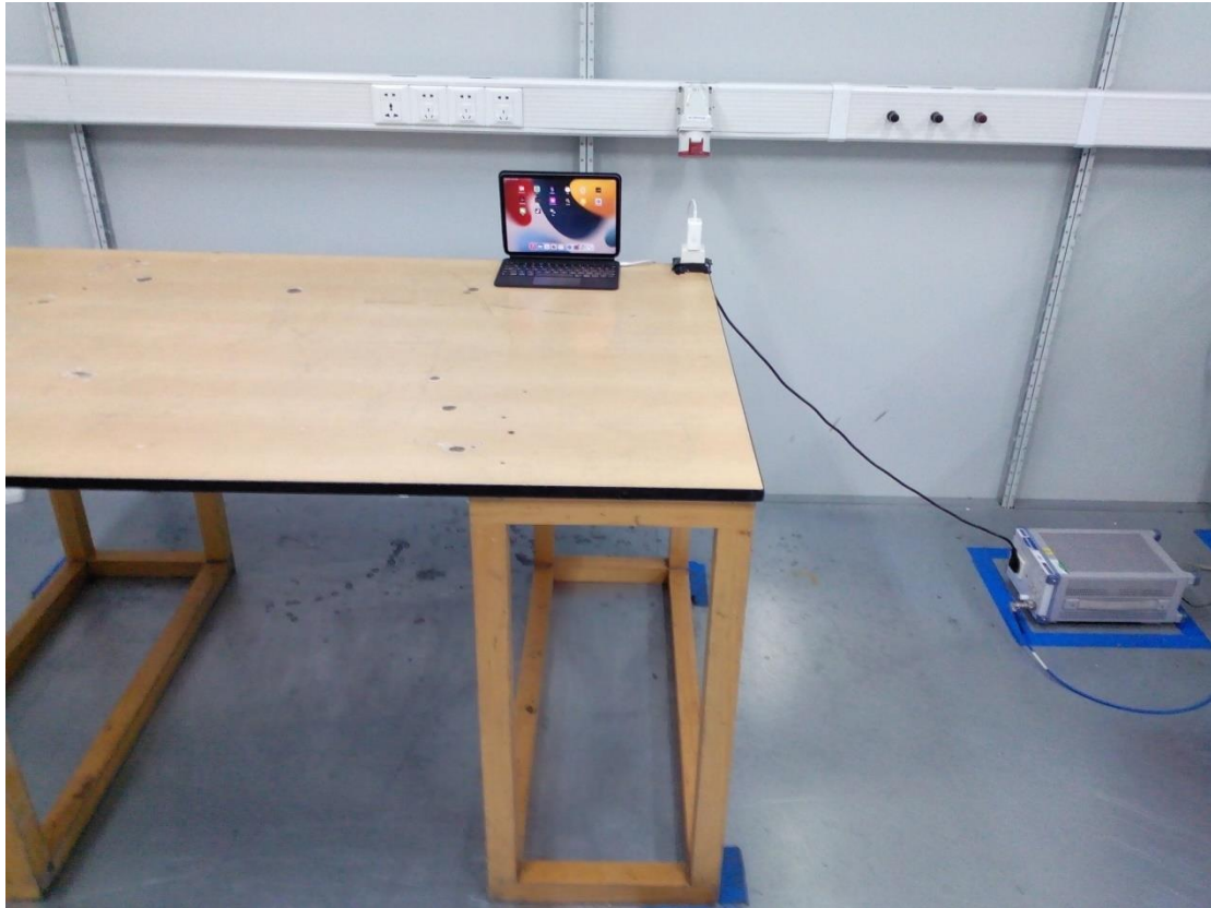
AC Conducted Emission Test Setup -Front
