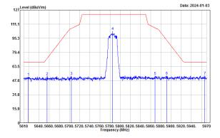
Site : LK-966A Condition: 3m vertical Mode : N20 TX-5785MHz Note : Temp/RH:19.1°C/64% Tester: Bruce
