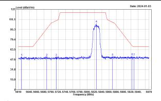
Site : LK-966A Condition: 3m vertical Mode : N20 TX-5825MHz Note : Temp/RH:19.1°C/64% Tester: Bruce
